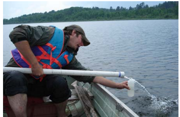
Filling a bottle with lake water to be tested for Phosphorus, & Chlorophyll .
