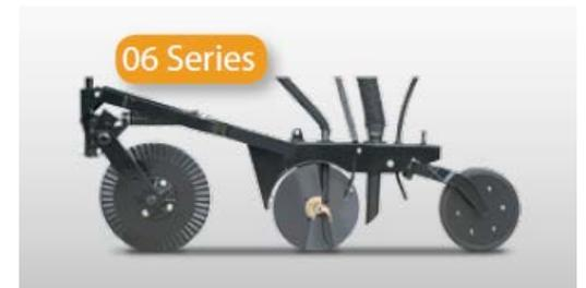
*View of opener assembly on the Great Plains 1006NT Drill. A turbo coulter is followed by an offset double disc opener and three inch wide middle ribbed packing wheel.*
